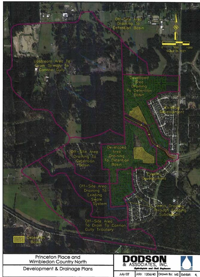
Figure 3: A significant portion of the area redirected drainage toward a new detention basin in the Wimbledon Falls development and then to the drainage channel.
