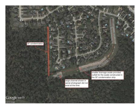
Figure 2: A drainage swale and berm was constructed along the western boundary.
