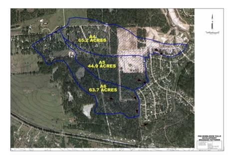
Figure 1: The Wimbledon Country storm drainage system that was designed in 1973 did not consider most of the 174 acres of off-site area draining toward it.
